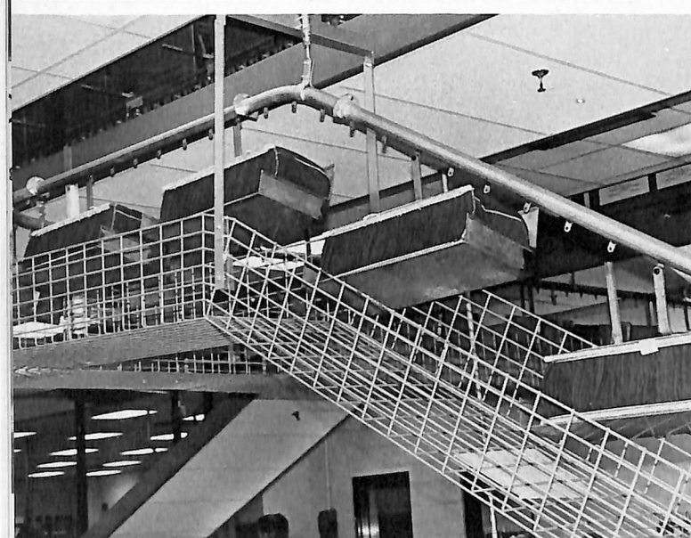
Top left: Crown Royal cases being emptied by the double-head uncaser. Current speed, about 14 cases per minute.
